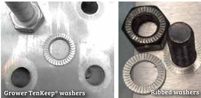
Figure 2: Internal test series – functional test: Grower TenKeep® washer versus other ribbed washer
