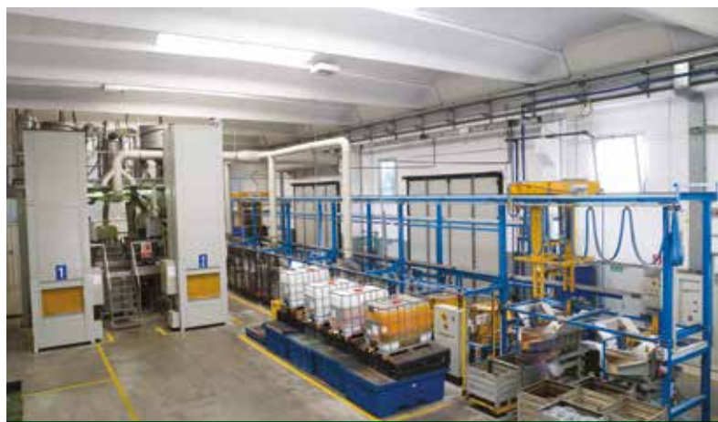
Growermetal's in-house zinc plating process
