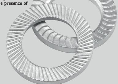
Grower Tenkeep safety washers are manufactured in three different versions – medium series (ideal for hexagonal head bolts), large series (ideal for flange headed bolts and for bearing surfaces made of soft materials such as aluminium, plastics, etc), and the cylindrical series (ideal for cylindrical head bolts). All three versions can be used with bolts of all strength classes up to 12.9.
